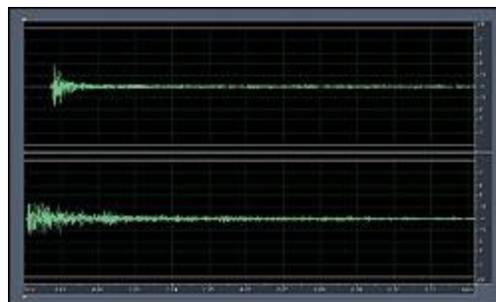
FIGURE 3a-b. Transient response for a high frequency (HF) microphone. Top (3a): Output from HF microphone.
