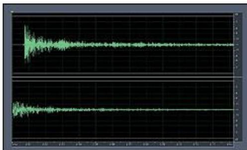
FIGURE 2a-b. Transient response for a broadband microphone. Top (2a): Output from a broadband microphone.
